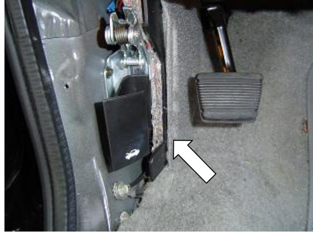
3. Peel the carpet back from the front left corner to expose the wiring that runs along the driver sill area inside the black plastic channels, and wedge the carpet under the brake pedal (or clutch pedal, if equipped).
