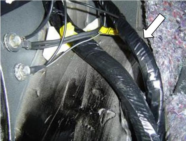
3. If you opened the black plastic channel next to the driver's side door sill, tuck the two wire bundles back into the black plastic wire channel and close the wire channel by squeezing the latch back into itself.
