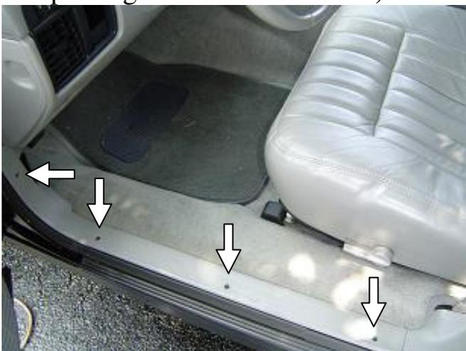
2. Remove/pull out the forward carpet trim piece (if it didn't come out with the door sill). This is the carpeted piece of plastic located to the left of the parking brake assembly.
