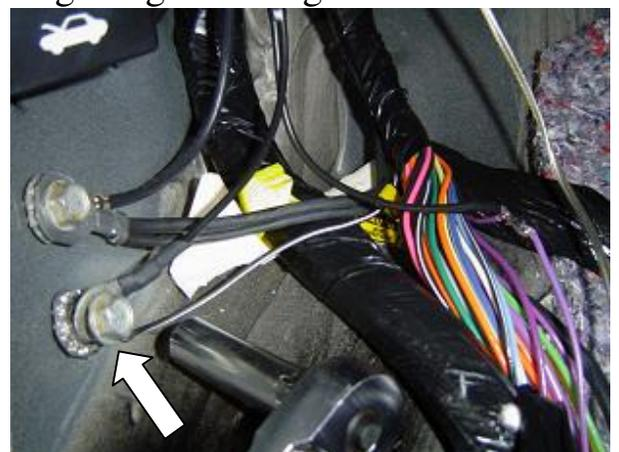
Alternate: Drill a pilot hole and make your own grounding point.
